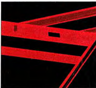
▲ Coordinated. Engineer ordered beam penetrations for duct runs.
